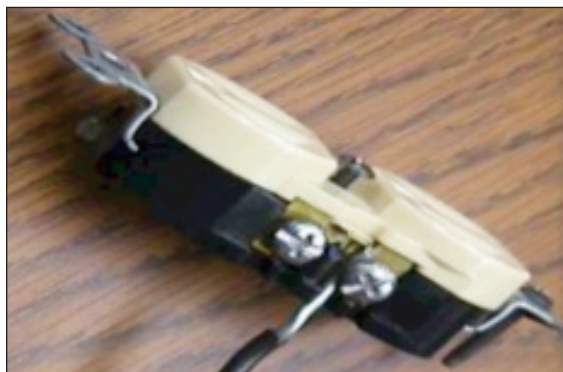
The fire shown in photo above started at the connections.
